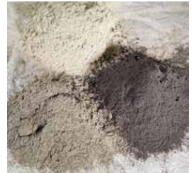
Figure 8a Fly ash, a byproduct of the electric industry, can be used as a partial replacement for portland cement.
