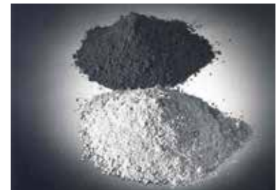
Figure 8c Silica fume, an industrial byproduct, is commonly used to replace cement in quantities from 5% to 7%.
